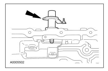
11. Install the manual valve inner lever onto the manual shaft and loosely install the nut.
